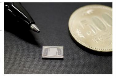
allow for nonmechanical, two-dimensional beam steering. A shallow-etched grating made into the photonic crystal waveguide was used as the double periodicity, increasing the upward emission efficiency. The team designed a bespoke prism lens to convert the steering angle in a desired direction, while maintaining the collimation condition for the steered beam.
